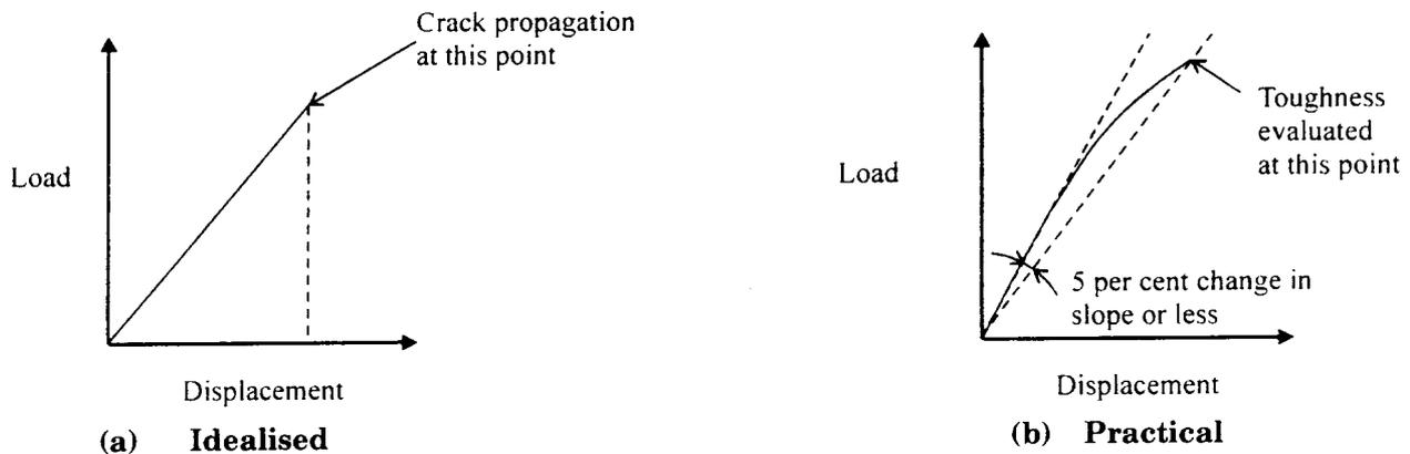
**Sketch 5.2 Local displacement curves obtained in tests for  $K_{Ic}$**
