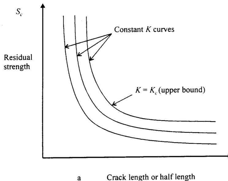
Sketch 5.5 Typical plots of residual strength versus crack lengths for constant  $K$
