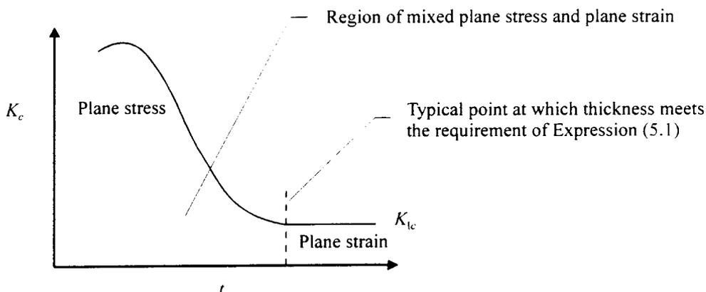
**Sketch 5.1 Typical form of relationship between fracture toughness and thickness**
