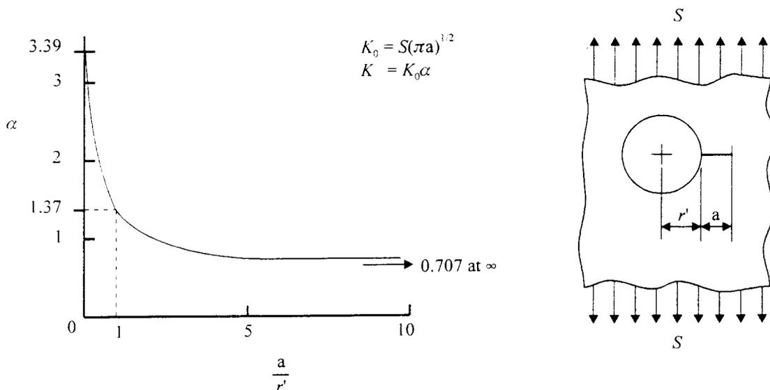
**Sketch 3.3** Illustrating a definition of crack length that does not include the local geometry
