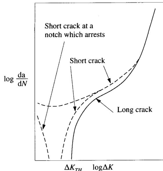
**Sketch 4.4 Comparison of the crack propagation rates of typical long and short cracks and for short cracks growing from a notch which arrests. All curves at a common value of stress ratio,  $R$ .**
